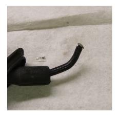
5. After a good dousing with alcohol, flatten the boot as shown in #1, and while flat....twist and push the old wire through as shown. Keep working it, it will come through. Note the tip is soldered in. I used a vise to hold the wire & heated the solder with a gun. Under that solder is nothing more than a small washer...remove it and use it on the new wire. Now pull the old wire back through the boot...may need more alcohol
