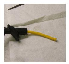
7. Douse the boot with more alcohol and pull the new wire back through until seated in the plastic case. Drop in the resistor and screw in the springy cap. Again, it's easier to move the wires in and out if the boot is flattened out...and don't forget the alcohol.
