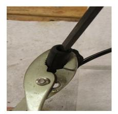
3. Unscrew the top piece (slotted for a screwdriver) by holding the internal plastic case firmly while still in the boot, but don't squeeze hard. It will come loose, but if you crack it do as I did with one...used some good plastic glue and let set overnight. It works fine. After removing the top screw-out piece, the resistor will drop out. Remember, the plastic case doesn't have to be removed.
