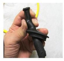
1. As stated above, flatten the boot with your hand as shown to enable moving the old and new wires in and out of the boot.
